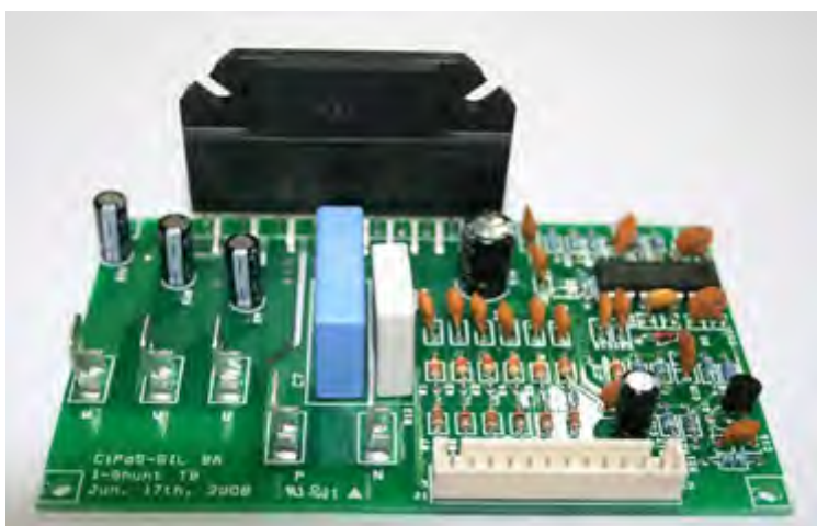
Figure 1 The picture of a reference board for CIPOS™ IKCSxxF60B(2)A
