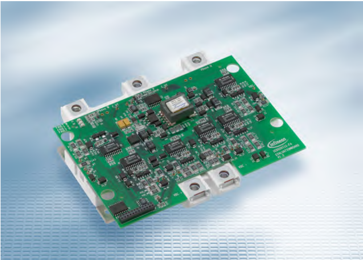
Figure 1 The 6ED100HP1-FA Evaluation Driver Board mounted on the top of the HybridPack1™ module
