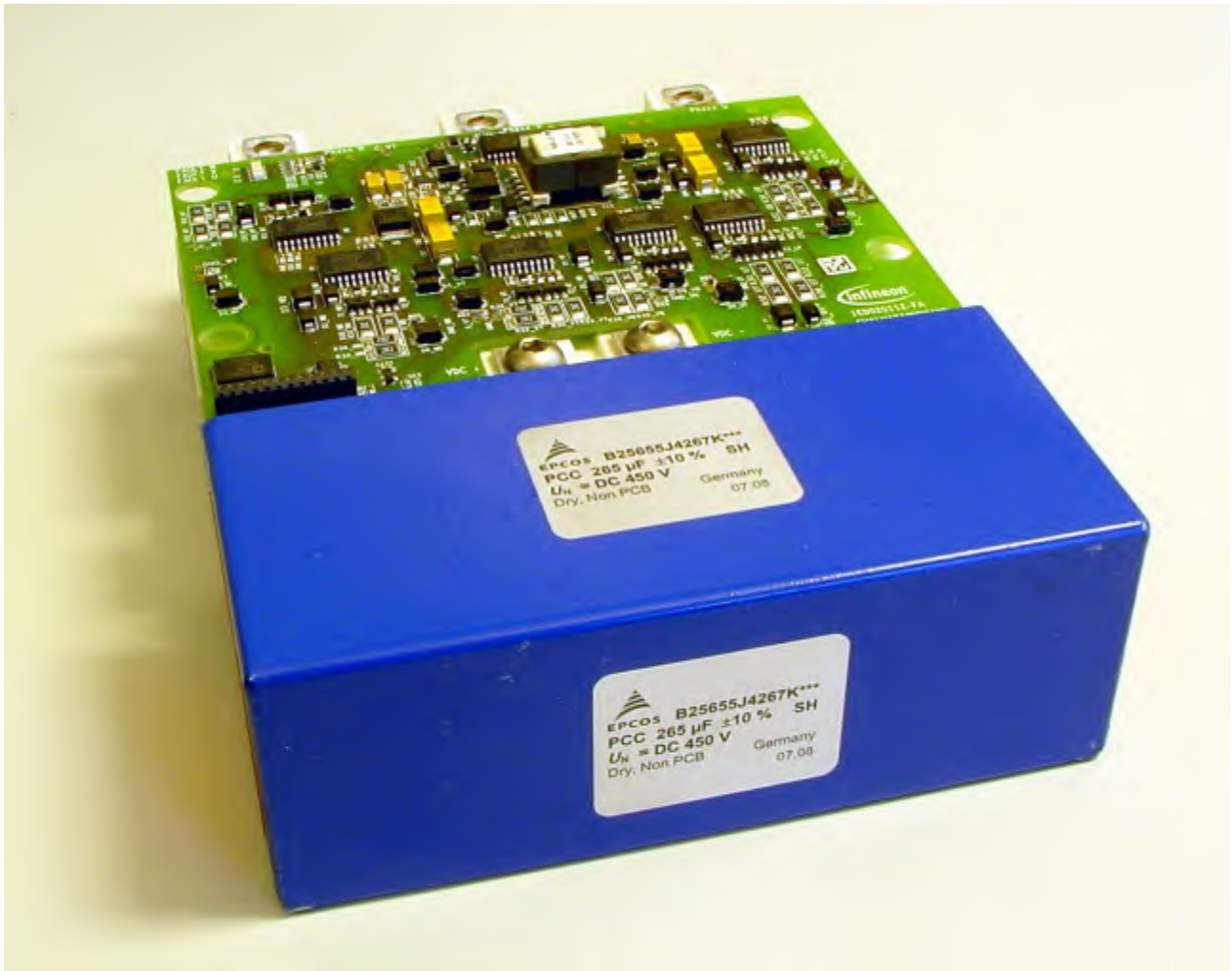
Figure 61 DC-Link capacitor screwed to HybridPACK™1 terminals
