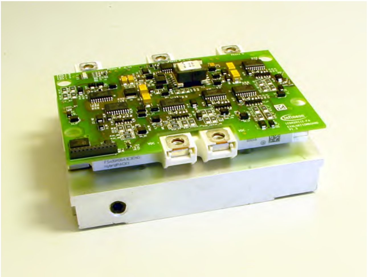
Figure 60 6ED100HP1-FA driver board on top of the HybridPACK™1
