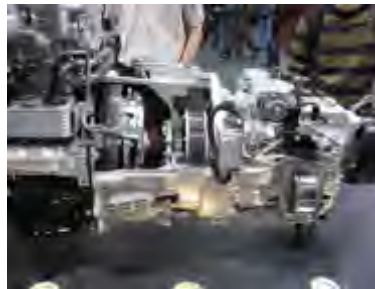
Parallel Power Train with PM machine Source: IAA2008, Mitsubishi Fuso
