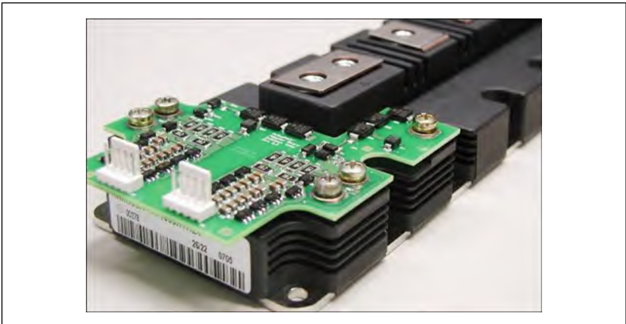
Figure 3 The MA300Exx correctly mounted on PrimePACK™ module
