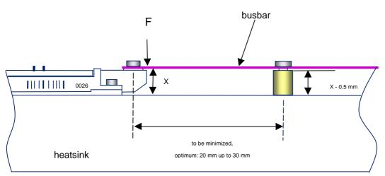
The power terminals can withstand this force F best in the direction from the terminal to the baseplate. Force to other directions has to be avoided. This has also to be considered in the tolerance of the busbar. See drawing as example for ideal mounting condition.
