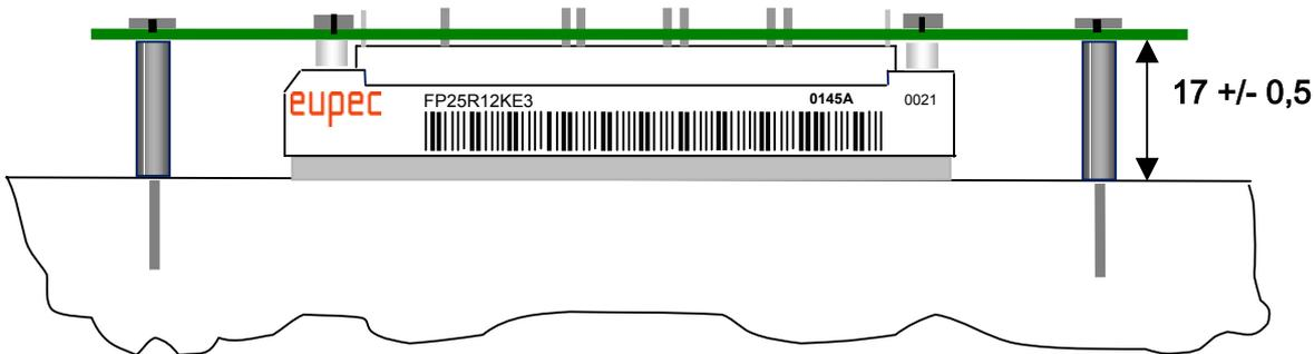
If more than one module is mounted on a PCB it is necessary to assure that the various base plates are on one level otherwise there will be mechanical tensions in the PCB which can destroy the construction..
