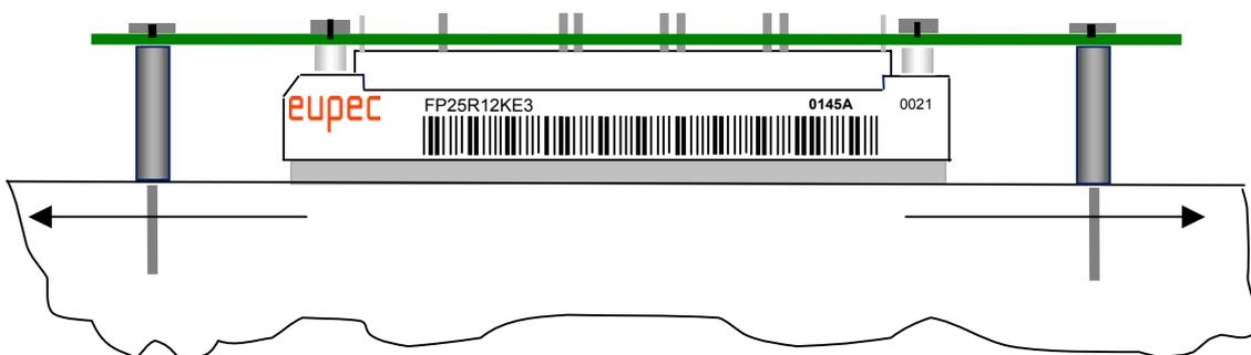
The pins can be desoldered with suitable facilities.
