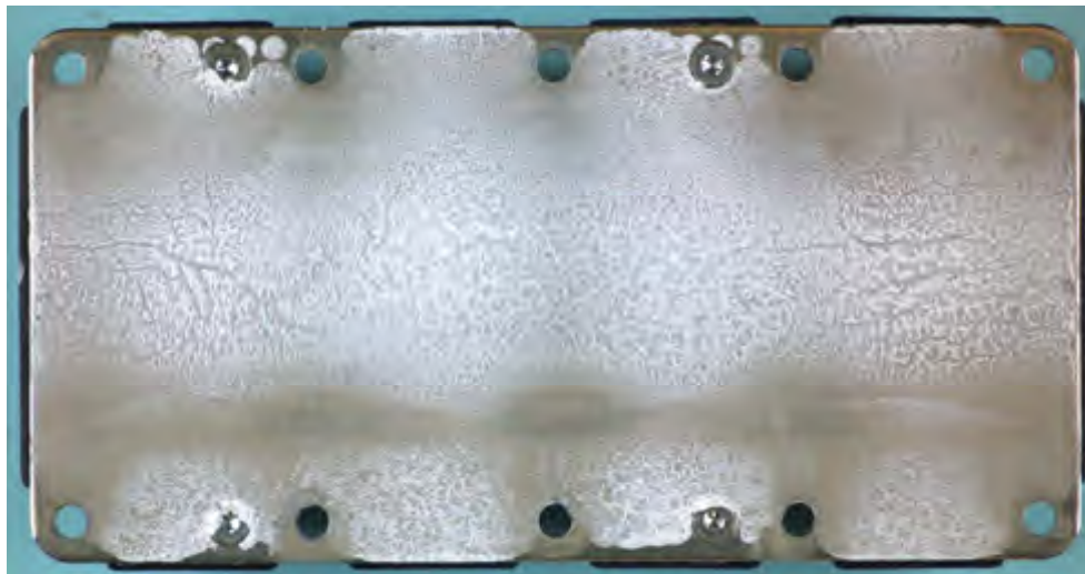
Figure 6 Base plate of the module with applied paste by screen printing after dismounting from heat sink.
