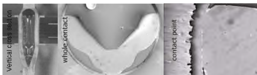
Figure 2: Easy PressFIT contact sections
