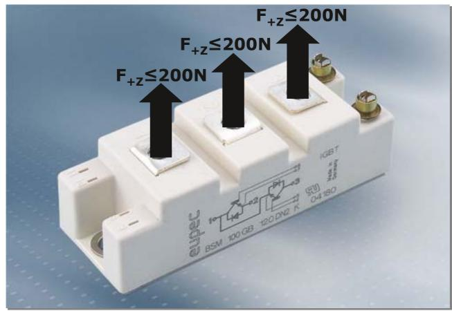
The modules must to be mounted in such way that the resulting pull-forces during mounting per power terminal of the module are limited to  $F+z\leq200N$ . Pulling, shocking and/or vibrational forces at the power terminals have to be avoided. The connection must be done in nontensional conditions.
