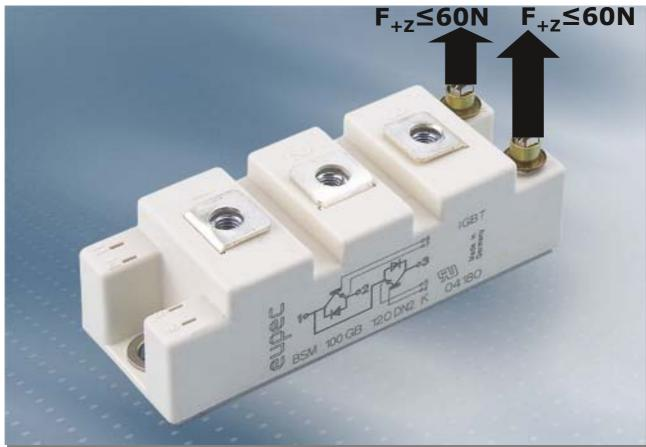
The modules must to be mounted in such way that the resulting pull-forces during mounting per control terminal of the module are limited to  $F+z \le 60N$ . Pulling, shocking and/or vibrational forces at the power terminals have to be avoided. The connection must be done in nontensional conditions.
