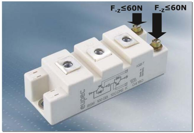
The modules must to be mounted in such way that the resulting push-forces during mounting per control terminal of the module are limited to  $F-z \le 60N$ . Pushing, shocking and/or vibrational forces at the power terminals have to be avoided. The connection must be done in nontensional conditions.
