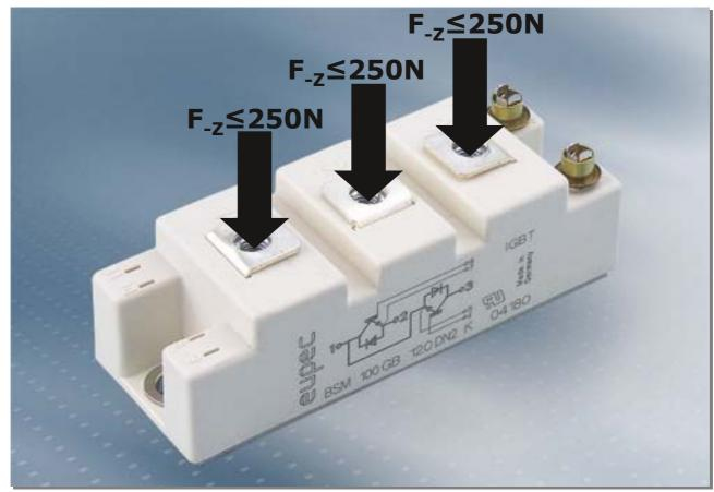
The modules must to be mounted in such way that the resulting push-forces during mounting per power terminal of the module are limited to  $F-z \le 250N$ . Pushing, shocking and/or vibrational forces at the power terminals have to be avoided. The connection must be done in nontensional conditions.
